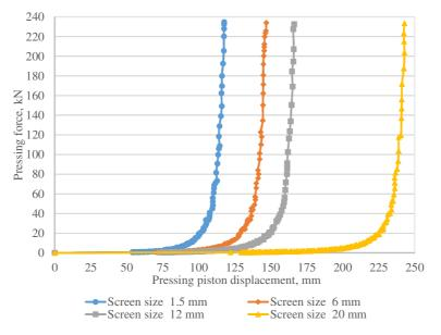
Fig. 4. Force – displacement characteristics of compacting
