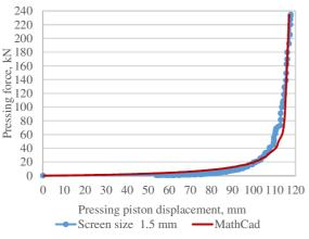
Fig. 5. Force – displacement (sieve 1.5 mm)
